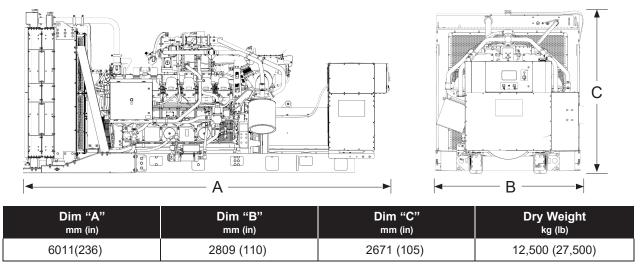
Note: For reference only. Do not use for installation design. Contact your local Cat dealer for precise weights and dimensions.
