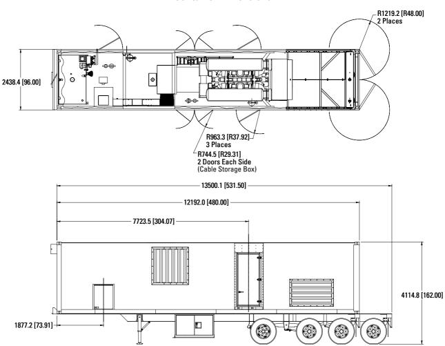
The power module must have support under the center when set on the ground.
