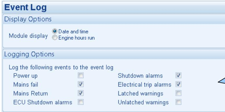
Example showing the possible configuration of the DSE7000 series event log (DSE Configuration Suite Software)
