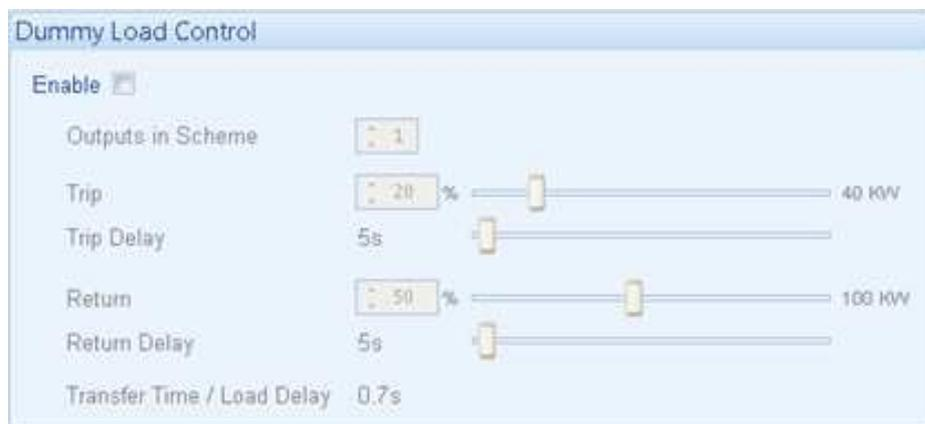
Example screen shot of *Dummy Load Control* setup in the DSE Configuration Suite
