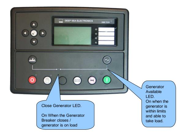
**NOTE:-** "Generator on load" LED has two modes of operation depending upon the configuration of the controllers digital inputs.
