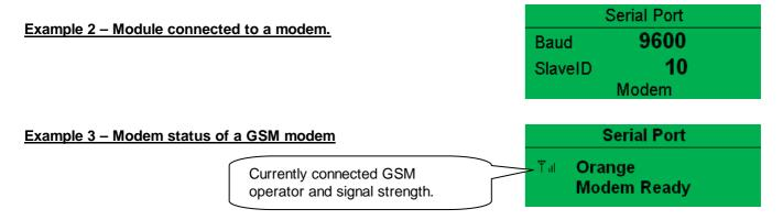
Many GSM modems are fitted with a status LED to show operator cell status and ringing indicator. These can be a useful troubleshooting tool.
