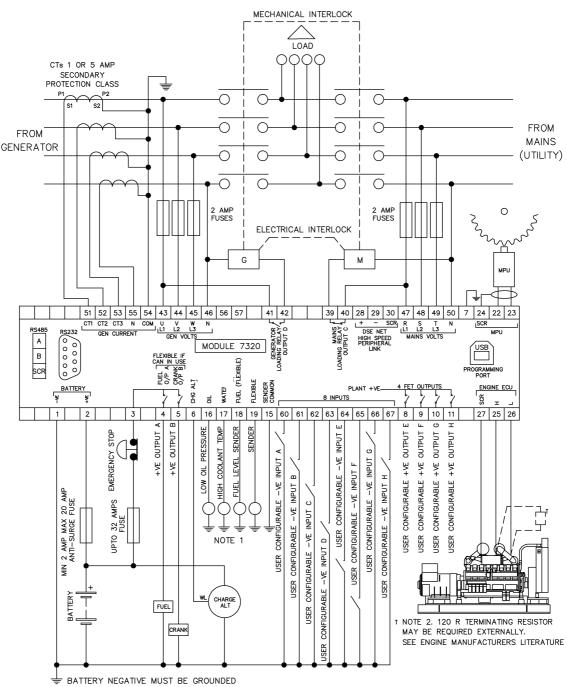
TERMINALS SUITABLE FOR 22-16 AWG (0.6mm - 1.3mm ) FIELD WIRING
