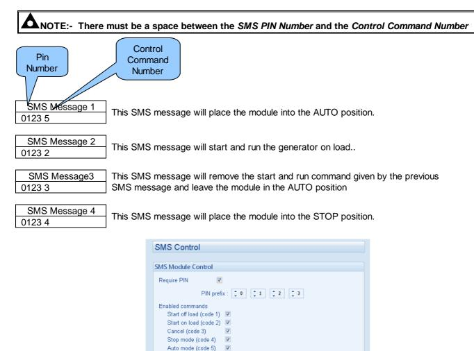
Example screen shot of SMS Control setup in the DSE Configuration Suite
