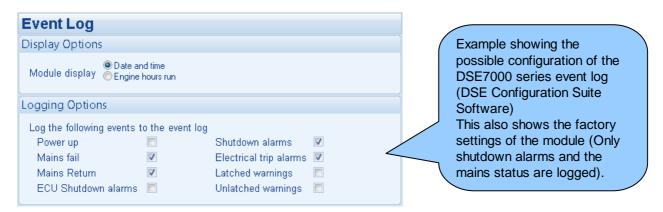
Once the log is full, any subsequent shutdown alarms will overwrite the oldest entry in the log. Hence, the log will always contain the most recent shutdown alarms.
