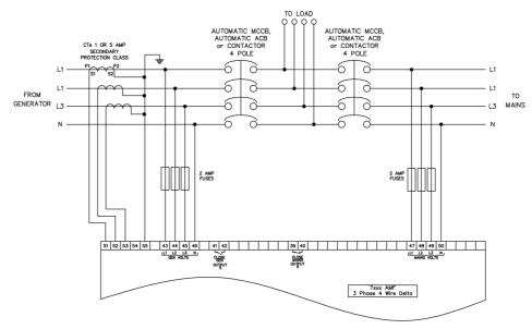
2) **Load**: The CTs are used to measure and display generator current when the generator is on load and mains current when the mains is on load. The module display automatically changes to display the current in the relevant instrumentation page. This example shows the CTs in the 'load' for a three phase delta system but the same philosophy is applicable to the other topologies.
