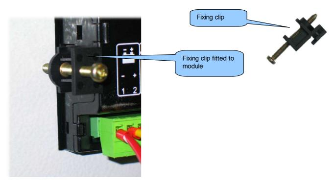
**O**NOTE:- In conditions of excessive vibration, mount the module on suitable anti-vibration mountings.
