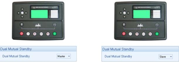
Screen shot from DSE Configuration Suite PC Software showing the configuration of the Master and Slave controllers.
