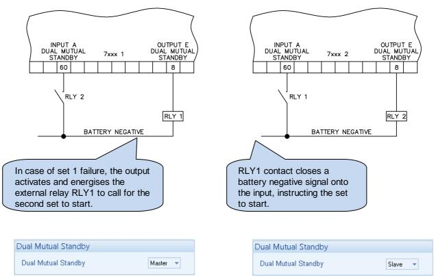
Screen capture from DSE Configuration Suite PC Software showing the configuration of the Master and Slave controllers.
