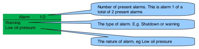
The LCD will display multiple alarms E.g. "High Engine Temperature shutdown", "Emergency Stop" and "Low Coolant Warning". These will automatically scroll in the order that they occurred.
