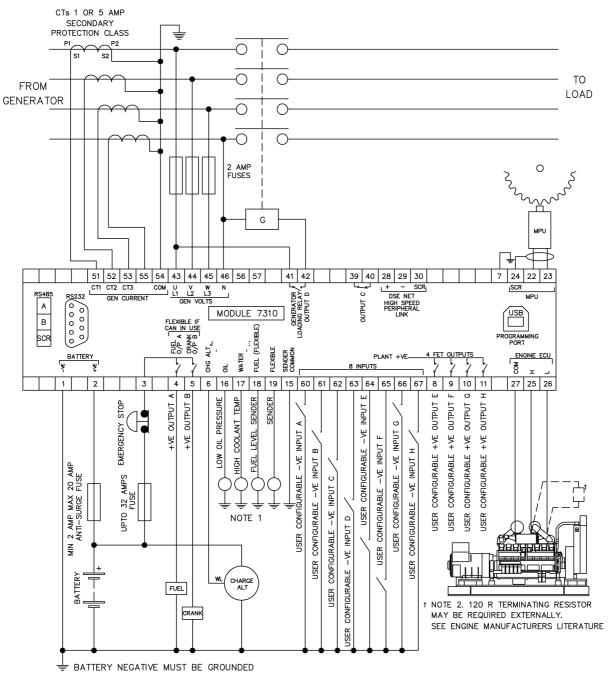
TERMINALS SUITABLE FOR 22–16 AWG (0.6mm – 1.3mm ) FIELD WIRING TIGHTENING TORQUE = 0.8Nm (7lb-in)
