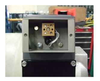
Fit a blind grommet to the cable entry side of the connection box.
