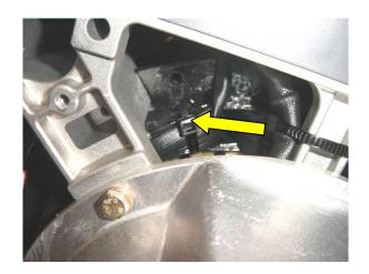
Pass the harness through the aperture in top of the NDE bracket, route it across to the grommet in the terminal box.
