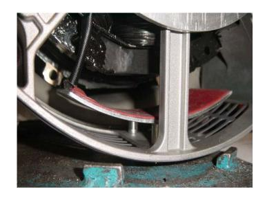
Secure the harness from the heater to the coil around the periphery of the exciter stator using a temperature resistant tie.
