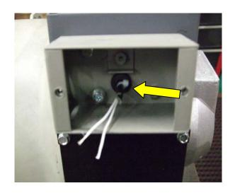
Insert the stripped lead ends into the terminal block and tighten the retaining screws ensuring that the contact is clamping onto conductor and not the insulator.
