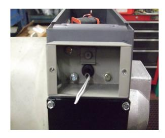
Trim the Systaflex sleeve so that it is 15mm proud of the grommet. Secure a cable tie around the Systaflex to ensure that it cannot be pulled back into the terminal box. Next, trim the leads so that they are 30mm proud of the end of the Systaflex and strip 5mm insulation from the end of each lead.
