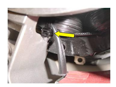
Secure the remaining harness to each individual coil around the periphery of exciter stator using temperature resistant ties
