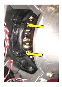
The cable which is now tied around the periphery of the exciter stator then exits at the 11.00 o'clock position.
