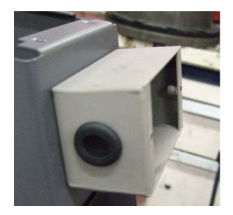
Fit a label showing the heater voltage requirement to the position shown in connection box.
