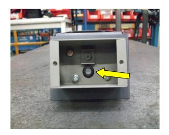
Feed the heater leads through grommet.
