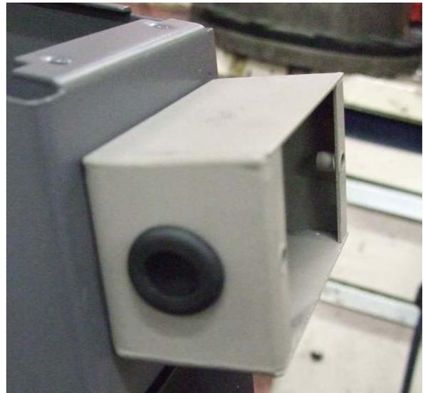
Fit a label showing the heater voltage requirement to the position shown in connection box.
