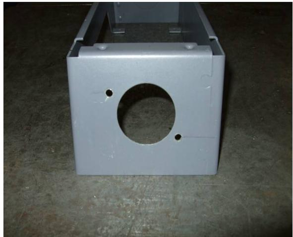
Fit the grommet to the hole in the heater connection box and secure the assembly to the terminal box using 2 off M5X12 hex head screws, spring washers and plain washers.
