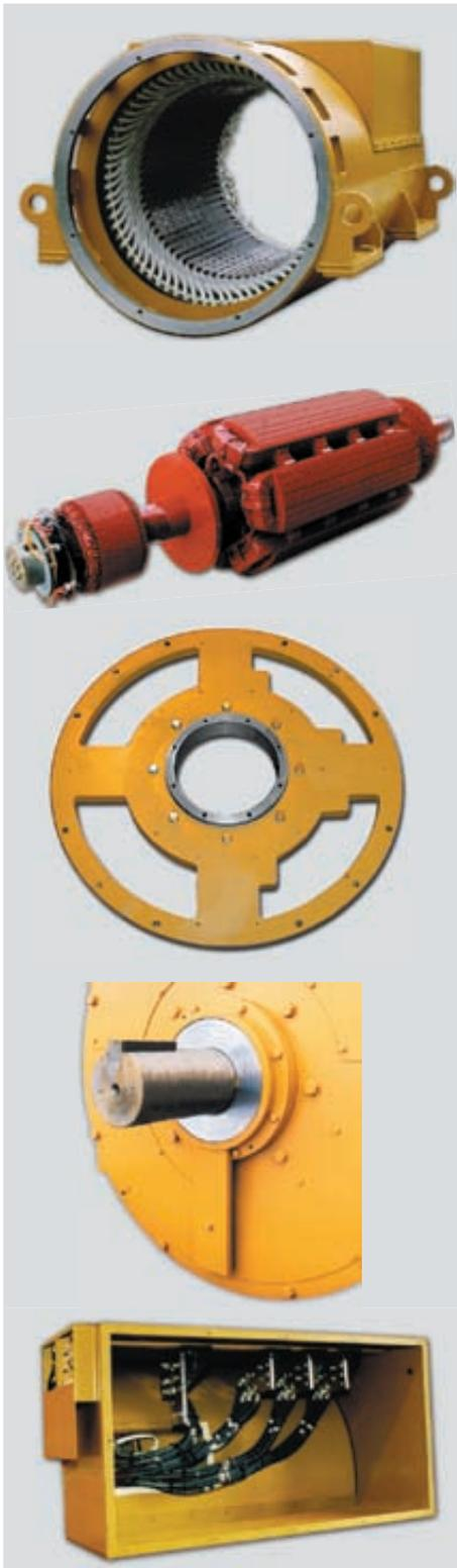
**Stator:** Kato uses Class H insulation for the stator with a Class B temperature rise for an efficient and compact generator with a long operating life. Mica turn taped magnet wire is used in the stator coils to provide nearly twice the instantaneous surge withstand capacity as glass-covered magnet wire.
